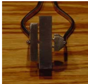
Other manufacturer's Tongs - Incorrect Fabrication results in Space between Tool and Specimen
