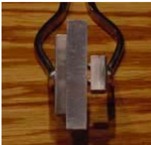
MPM Tongs - No Space between Centering Tool and Specimen
