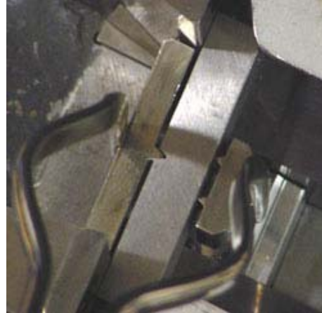
Other manufacturer's Tongs - Tool is Past Anvil Radius when Specimen is Deposited
