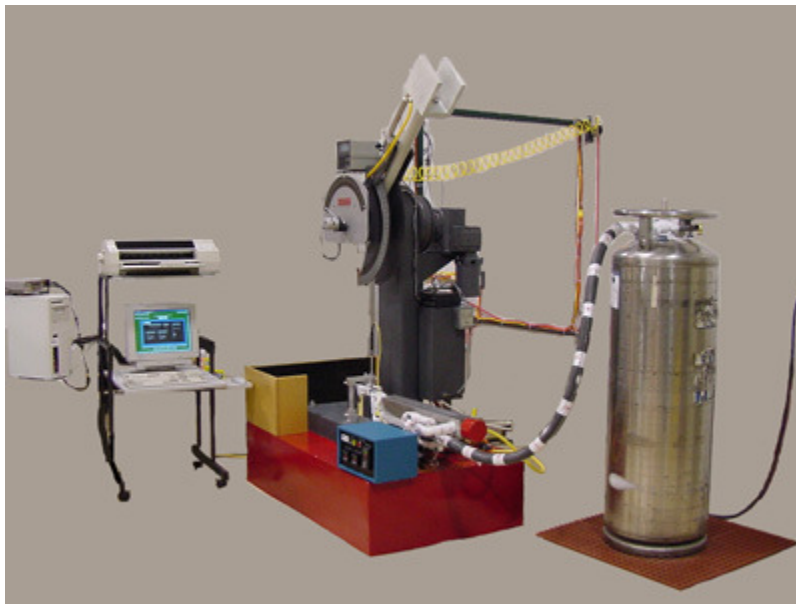
Tinius Olsen Model 84 Pendulum Impact Test Machine equipped with in-situ heating and cooling system, optical encoder, and motorized hammer return.
