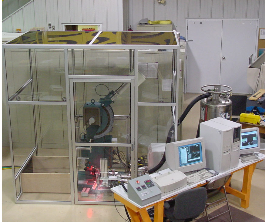
Automatic Charpy machine with Specimen Transfer System, In-Situ Heating/Cooling, Specimen ID Reader, and Computer Control System.
