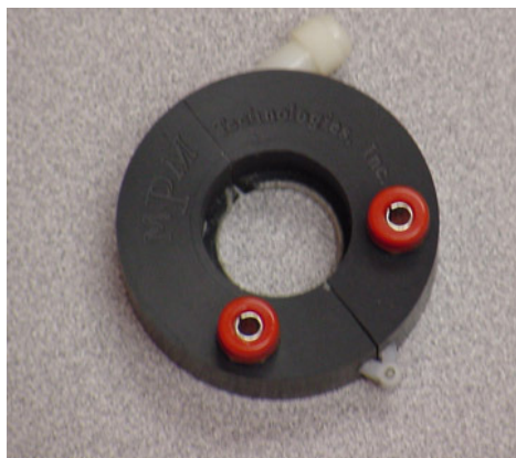
Dry reference electrode for electrochemical measurement of components which would be damaged by exposure to a wet reference electrode.
