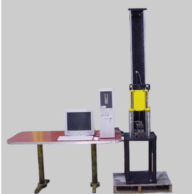
Refurbished drop tower equipped with state-of-the-art instrumented striker system.
