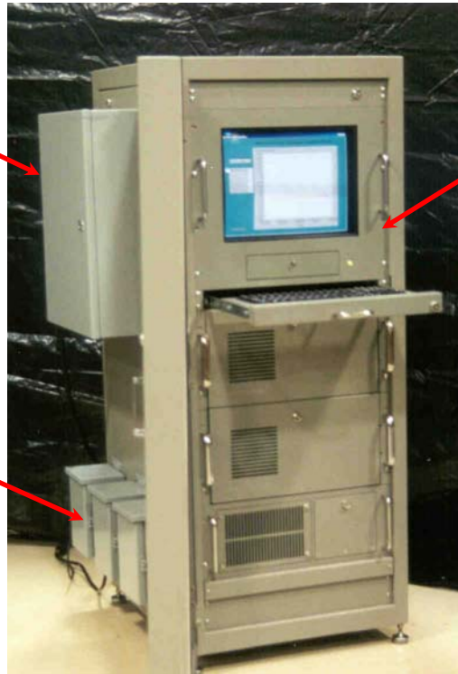
Data Acquisition and Control Cabinet with Off-Site Data Transfer Capability
